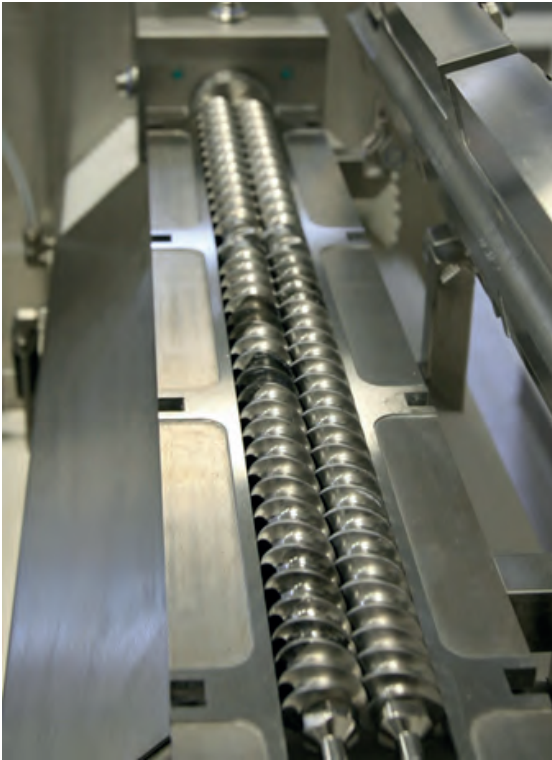
Fig. 2: Insight into the process zone of the granulator, which is part of the QbCon® 1.
